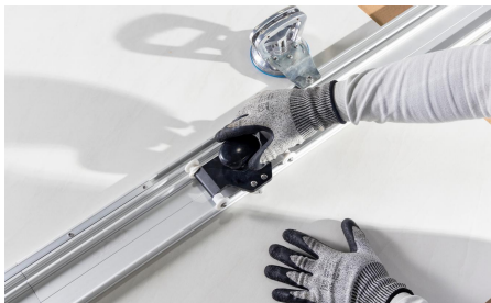
Image 62: Fit the wheel onto the rail
