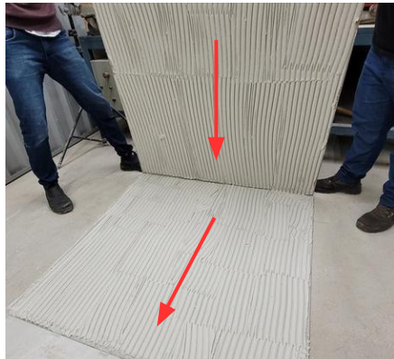
Image 29: Open mortar grooves in the same direction.
