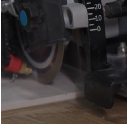
Image 75: Cut only into the surface layer of the varnish.
