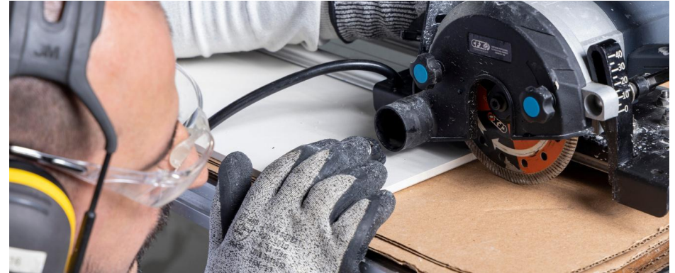
Image 73: Check that the disc is in the cut location.
