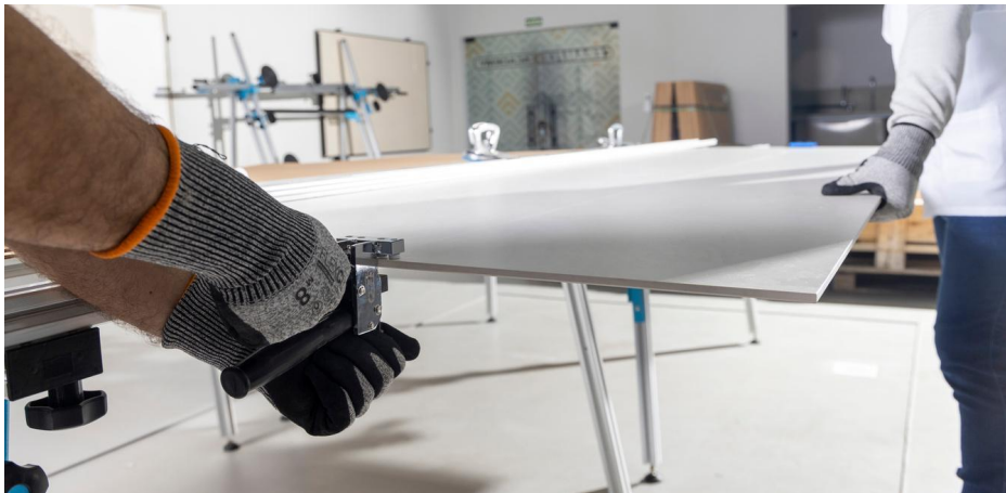
Image 67: On one side, turn the handle of the pliers until the score is partially open.
