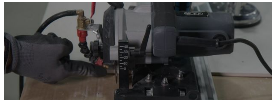
Image 74: Adjust the lever according to the cut depth.
