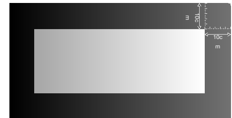
Image 20: Cutout to fit the fireplace at least 10cm from the edges/sides.
