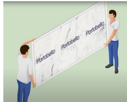
Image 06: Correct handling of slabs.
