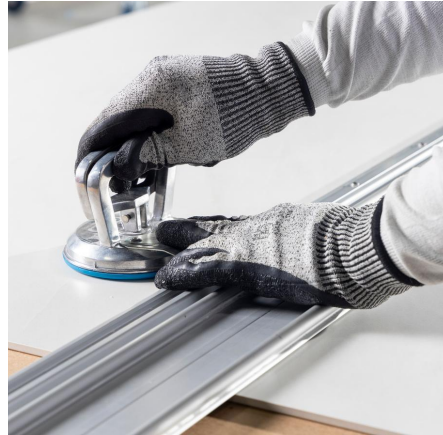
Image 71: Fix the rail with a suction cup to the piece.
