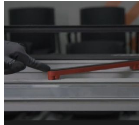
Image 50: Adjust the scorer's side support rods, according to the size of the piece.
