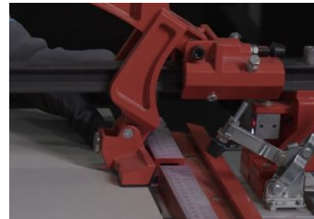
Image 56: Position the scorer foot at the end of the piece, applying pressure.
