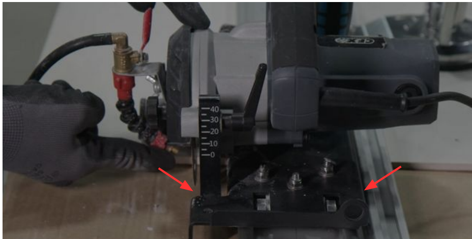
Image 72: Sliding accessory attached to the marble saw.
