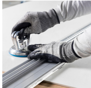
Image 61: Fix the rail to the piece with a suction cup.
