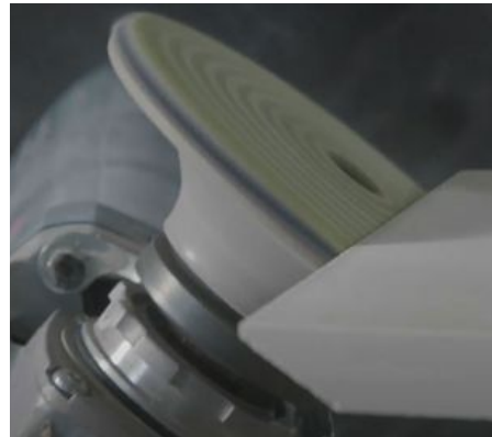
Image 99: Finalizing the removal of the outstanding 2mm with a ceramic disc.
