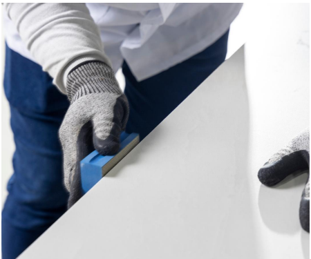
Image 100: Use of diamond sanding pad for fine finishing.
