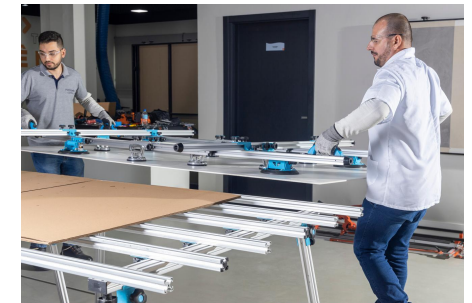
Image 93: Moving the piece to the covered cutting table.
