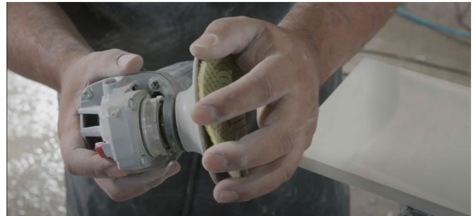
Image 102: Attaching the ceramic disc to the grinder.
