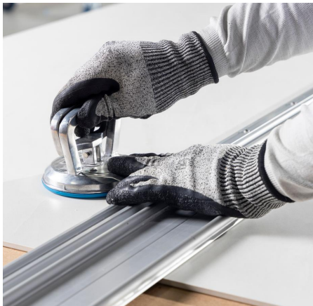
Image 94: Fix the rail to the piece with a suction cup.
