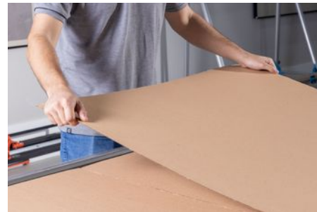
Image 92: Covering the cutting table with cardboard.
