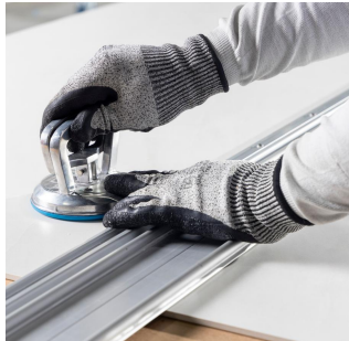
Image 61: Fix the rail to the piece with a suction cup.
