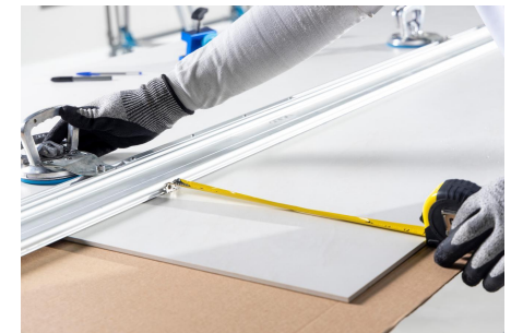
Image 59: Marking the rail fitting
