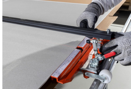
Image 53: Adjust the diamond blade of the scorer to the marking.
