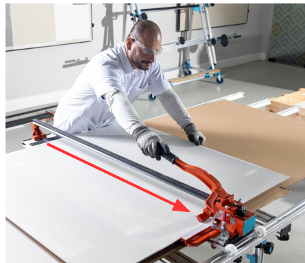
Image 55: Complete the score by pushing the diamond blade from one end to the other.
