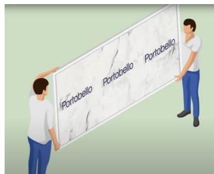
Image 06: Correct handling of slabs.
