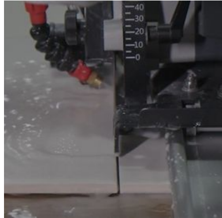
Image 76: Cut directly through the depth of the product.
