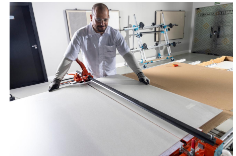
Image 57: With the pressure of the foot on the piece, the score will break.
