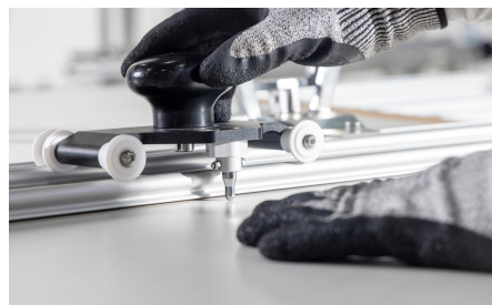
Image 63: Check that the scored area fits on the cutting area.
