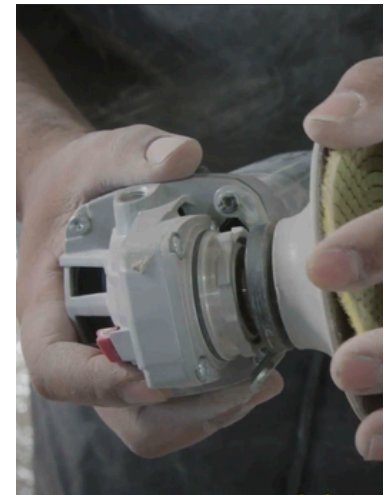
Image 102: Attaching the ceramic disc to the grinder.
